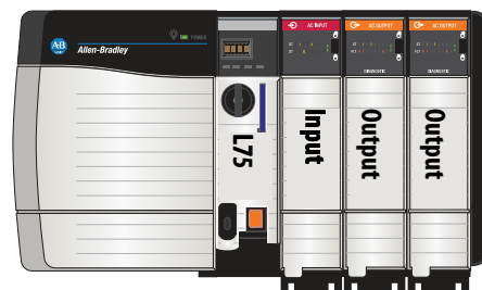
Figure 7 - Standalone Controller and I/O5
